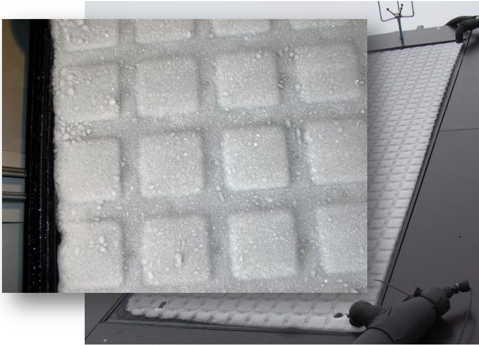
Figure 8: Frost on an uncovered solar collector operated below the dew point (source: SPF).
